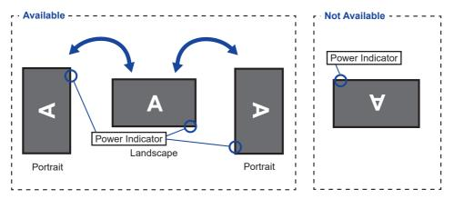
This model does not have a rotation mechanism, but the monitor can be rotated if use without Stand.
